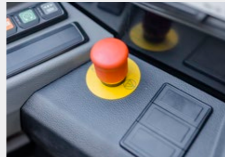
Quick-to-reach emergency button, so that the machine can be immediately put into a safe state in an emergency.
