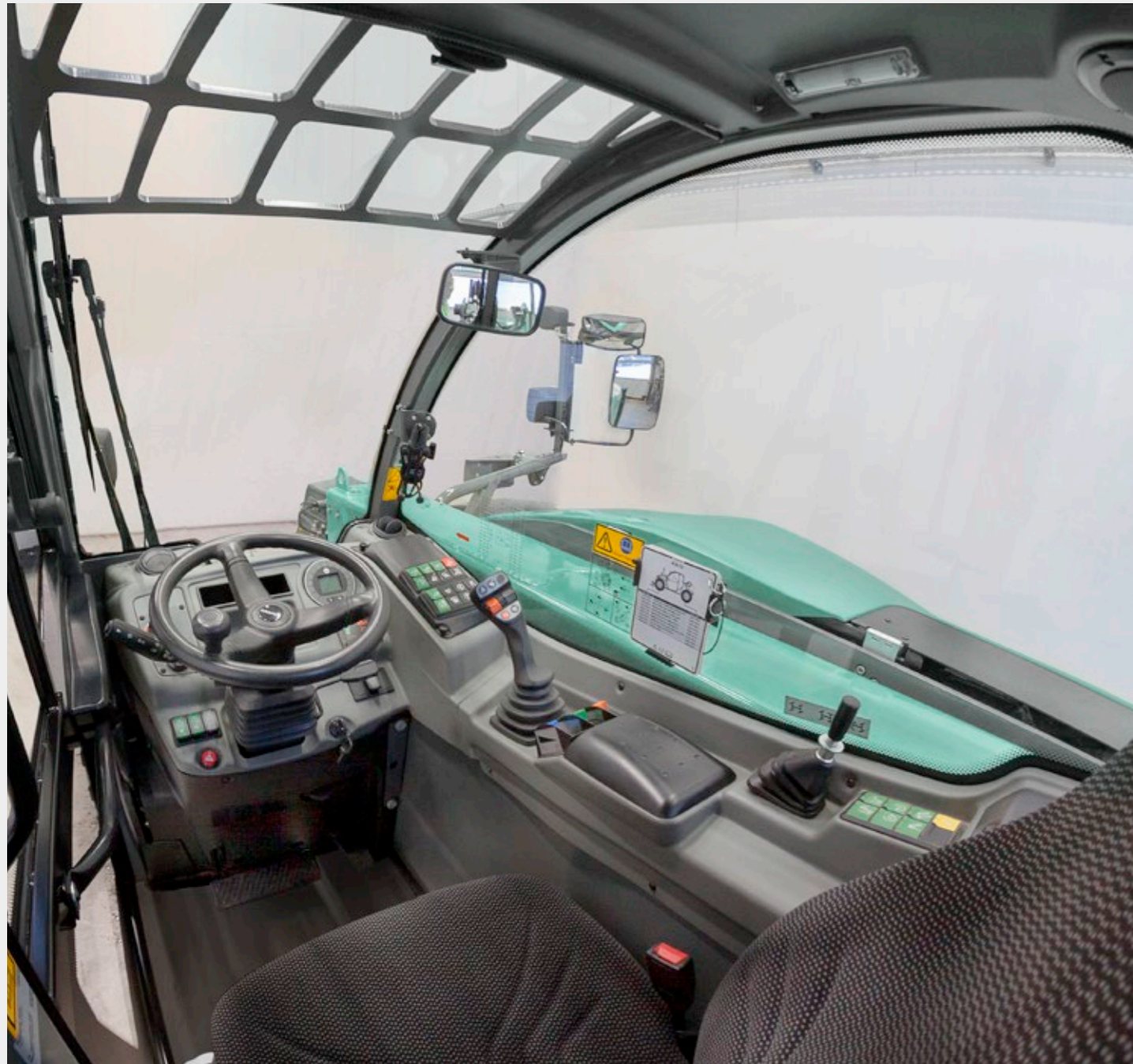
Good visibility to the right due to the large dimension, right window and low position of the telescopic boom.
