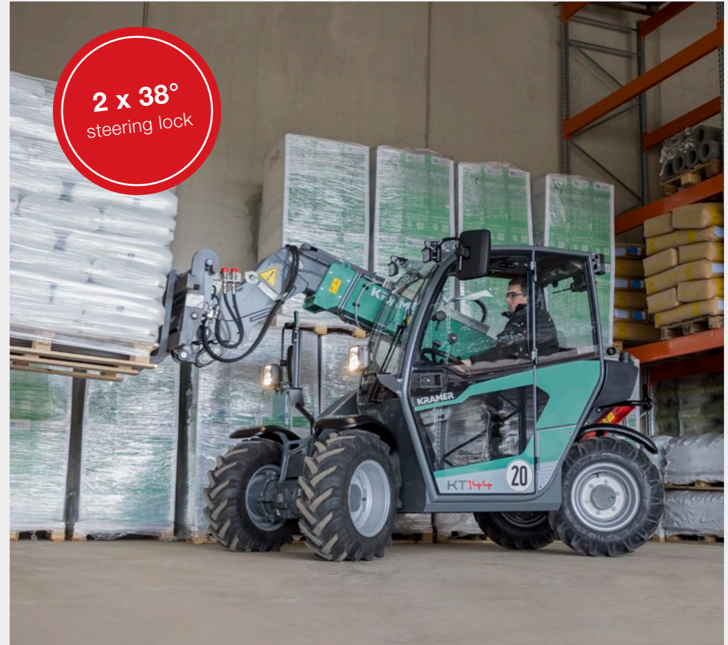
All-wheel steering: particularly manoeuvrable in tight spaces
